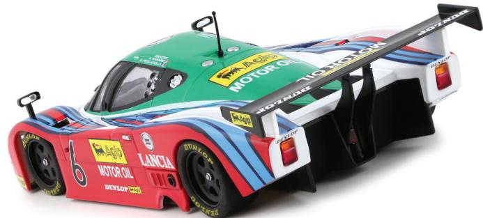
The wheels diameter was 15 inches at the front and 17 at the rear. Chassis was made of aluminum and magnesium; body material was carbon fibre composite.
